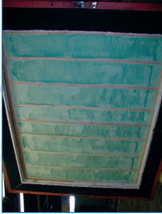
ASTM C1363: Interior side of SPF test wall
