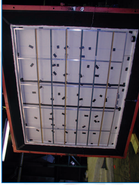
ASTM C1363: Interior side with gypsum wallboard and thermocouple grid
